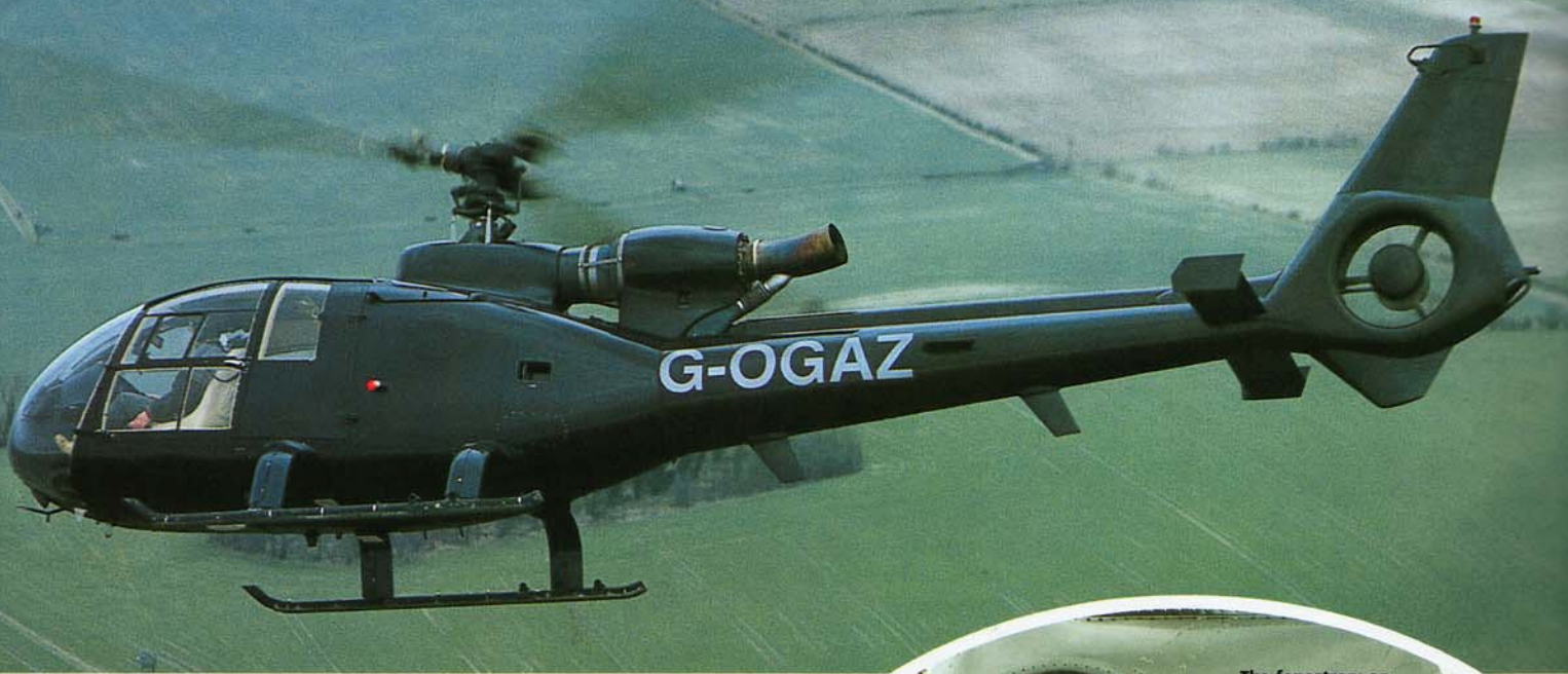
The fenestron: an unusual design and a source of both criticism and praise
